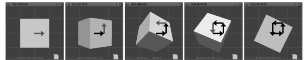
Figure 10: A conventional rotation technique: The final position is different from the initial one.
